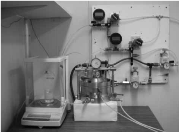
Figure 1. Experimental setup for suction controlled oedometer tests.
