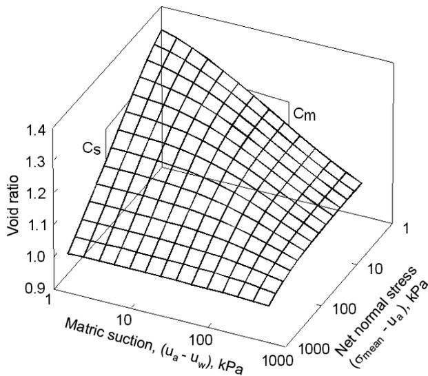
Figure 2. A typical void ratio constitutive surface
