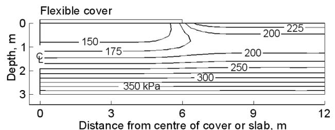
Figure 7. Contours of matric suction after three days of evaporation
