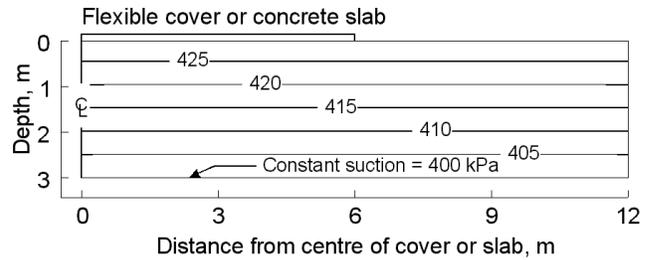
Figure 11. Initial matric suction condition for edge lift mode of analysis
