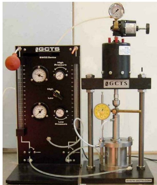
Figure 2. Photo of the GCTS pressure plate apparatus for measuring water content and volume changes in unsaturated soils under simultaneous control of total stress and matric suction.
