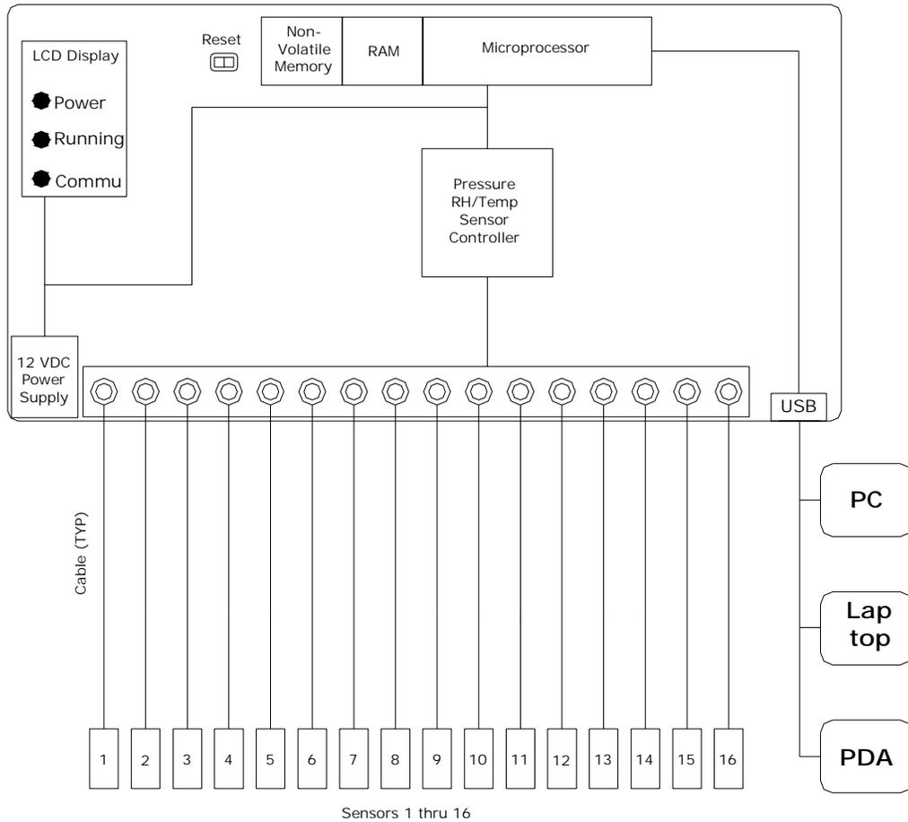
**Figure 5. A schematic of the GCTS datalogger.**
