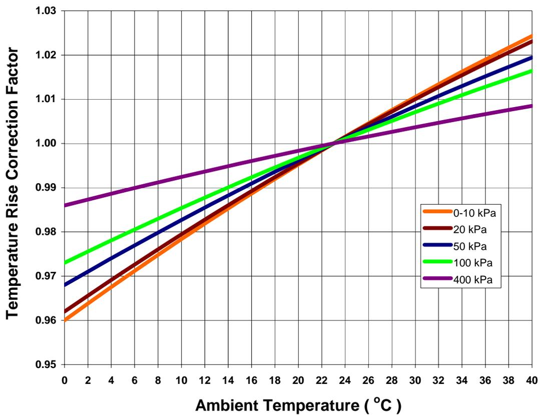
Figure 7. Correction factor for ambient temperature (Nichol et al. 2003).
