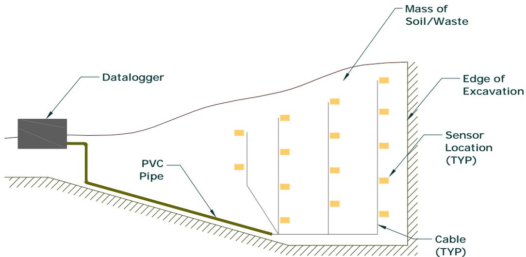
**Figure 4. A sensor installation layout (Tan et al. 2003).**
