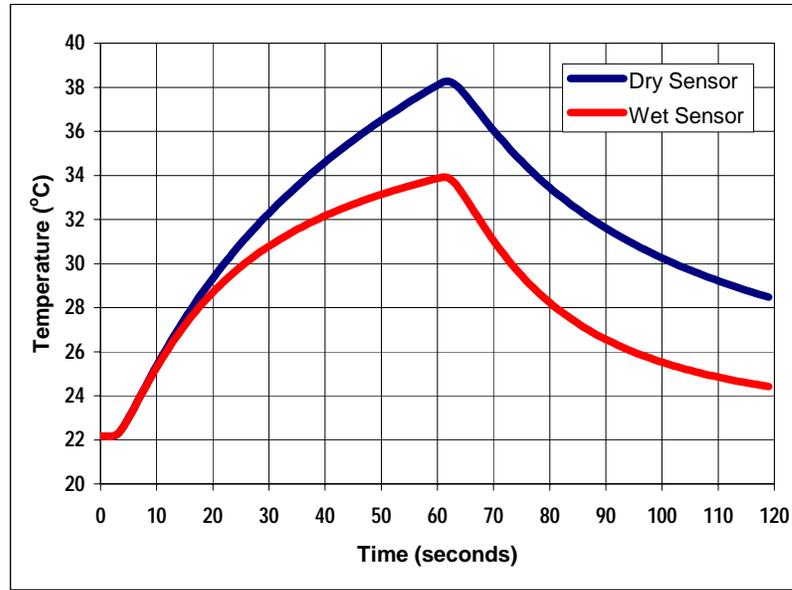
**Figure 2. Heating curves showing temperature rises in wet and dry sensors.**
