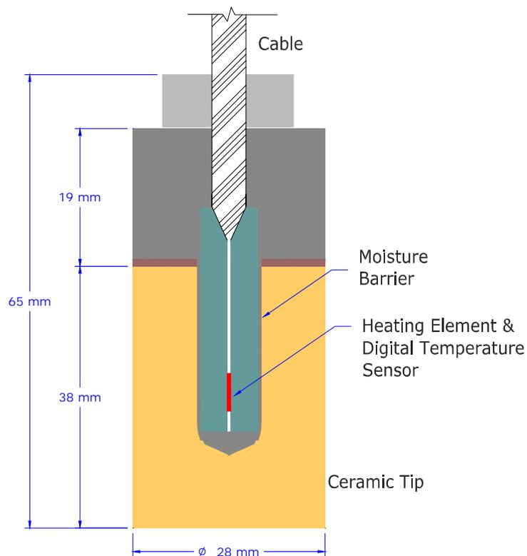
**Figure 1. Cross-section of Fredlund Thermal Conductivity Sensor.**
