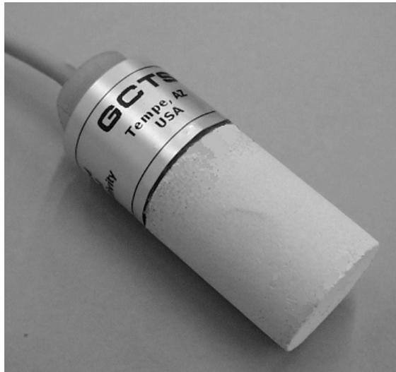
**Figure 3. Photograph of FTC sensor.**
