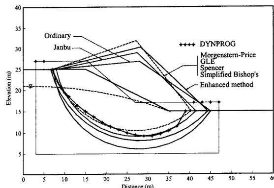
Figure 3. Solution of example 1 obtained by various methods.
