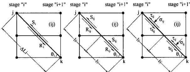
Fig. 2. Auxiliary function calculated from elemental shear strength and shear stresses.
