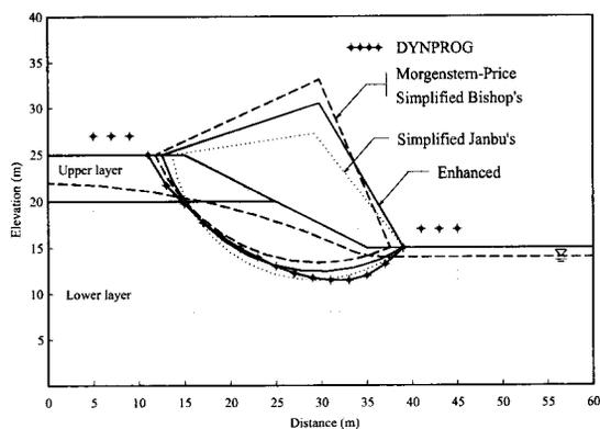
Figure 4. Solution of example 2 obtained by various methods.
