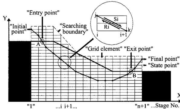
Fig. 1. The analytical scheme of the slope stability analysis using DP technique.
