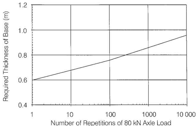
the known material properties. The bearing capacity of the pavement was obtained by varying the depth of the base layer until the calculated bearing capacity became equal to the equivalent contact pressure given by [6]. Single axle loading with single tires was assumed.
