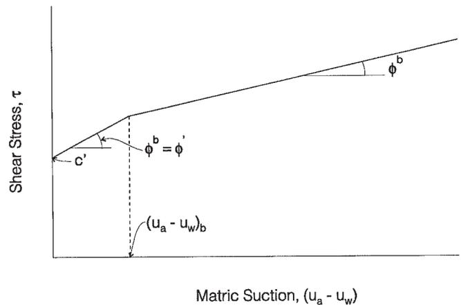
suction can be visualized as a contribution to the cohesion of the soil, and the components of the equation for the shear strength of the unsaturated soil can be rearranged as follows:
