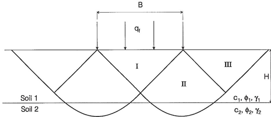
considers the base layer as an elastic material whose sole purpose is to distribute the load to the subgrade (Broms 1963, 1964; Bender and Barenberg 1978; Giroud and Noiray 1981; Milligan et al. 1989; Sattler et al. 1989; Szafron 1991). The second method assumes a general shear failure type of mechanism involving all pavement layers (McLeod 1953).
