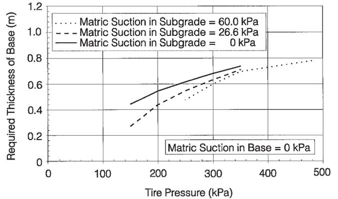
**Fig. 11.** Required thickness of the base layer versus tire pressure for different factors of safety for a static axle load of 300 kN.
