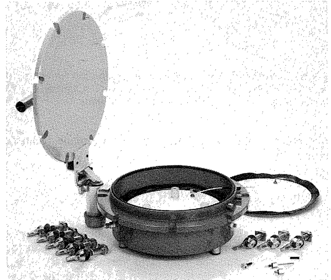
FIG. 9. 15 bar ceramic-plate extractor (i.e., maximum applied matric suction is 1500 (kPa) (photography courtesy of Soilmoisture Equipment Corporation, Santa Barbara, Calif.).
