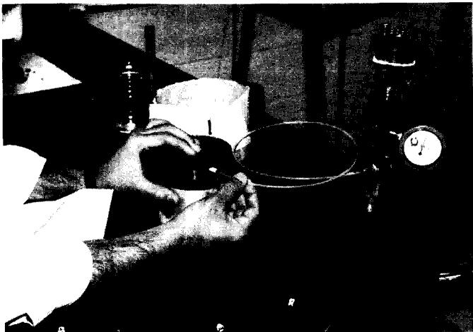
FIG. 6—Installation of the tensiometer tip into the Type II oedometer ring.
