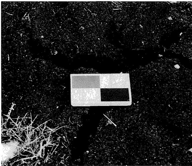
FIG. 10. An example of fissured Regina clay.
