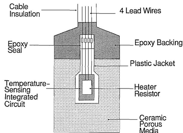
FIG. 1. A cross-sectional diagram of the thermal conductivity sensor.
