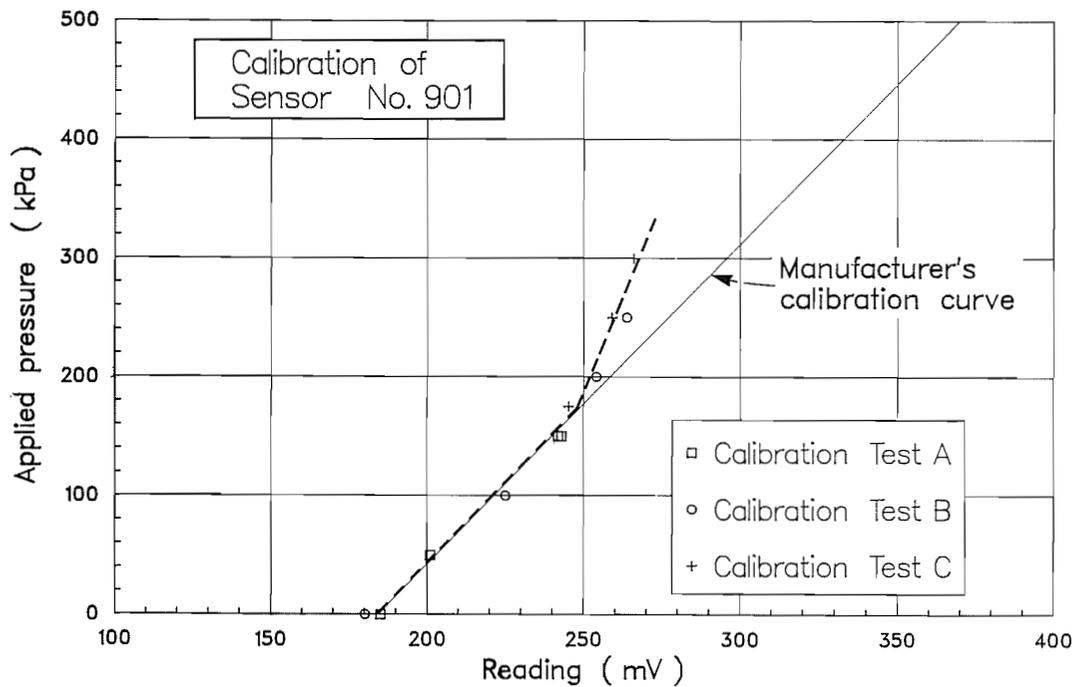
FIG. 3. Repeated calibration for sensor No. 901.
