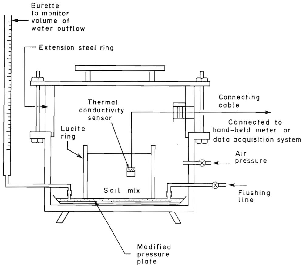
FIG. 2. Pressure plate calibration of thermal conductivity sensors.
