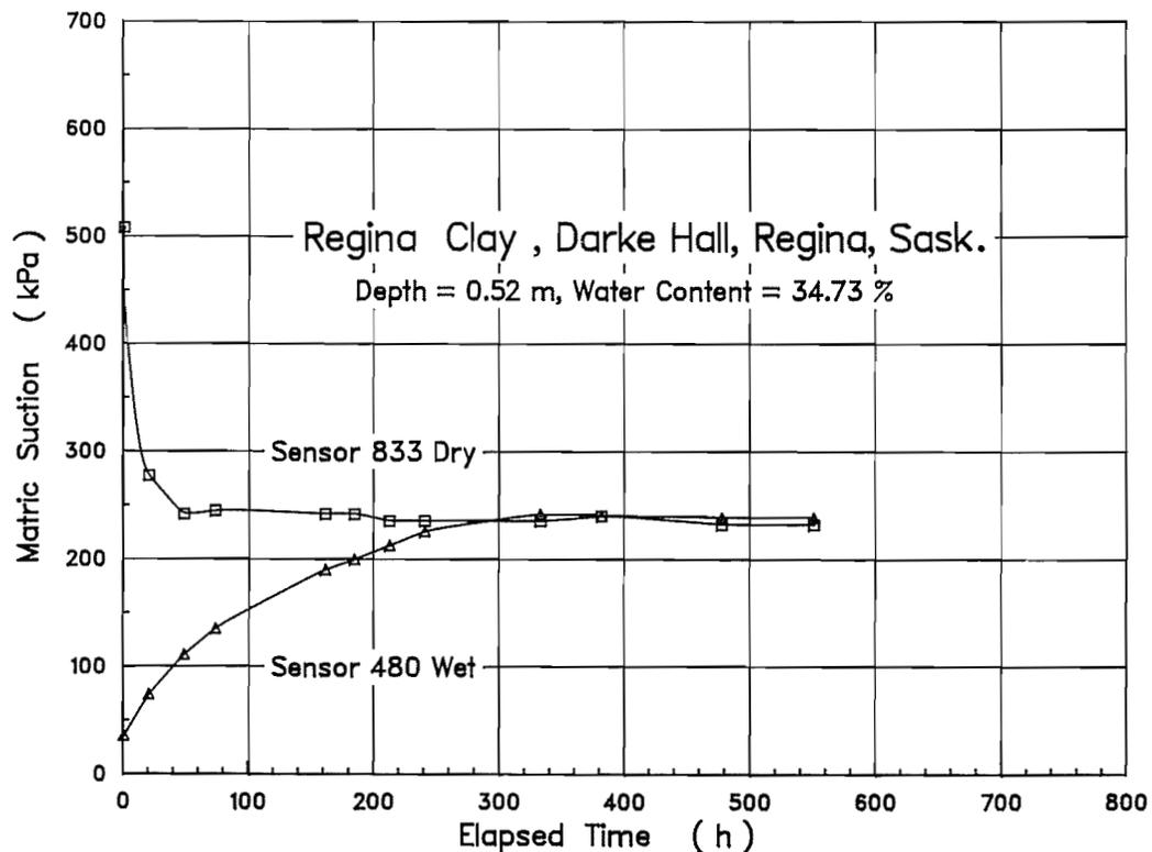
FIG. 7. Matric suction equalization for Regina clay.
