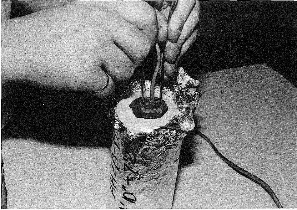
FIG. 4. Installation of a thermal conductivity sensor.
