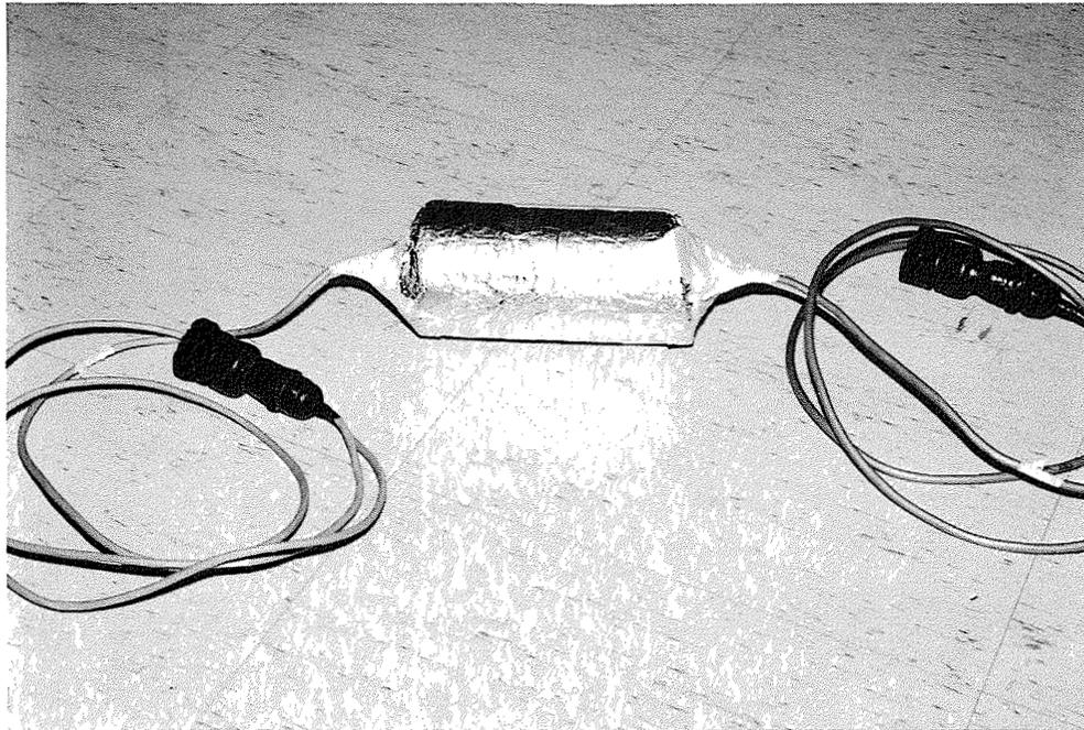
FIG. 6. A completely sealed sample with two thermal conductivity sensors installed.
