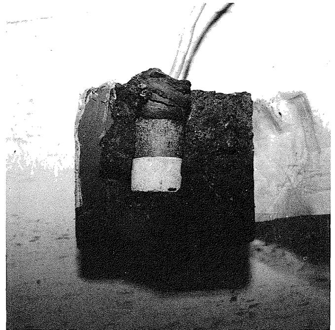
FIG. 5. Illustration of good soil-to-sensor contact.
